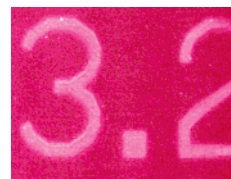
Figure 4. Two-photon photolithography (800 nm) using Novolac-diazonaphthoquinone-based photoresist. The size of the image is 3 \times 2 \text{ mm} .
